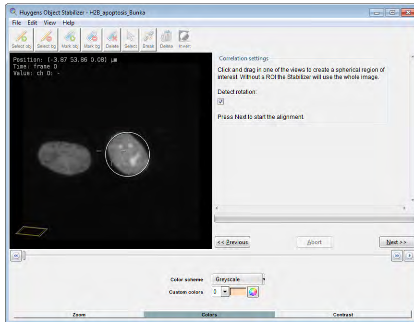
FIGURE 21.1. The Correlation settings screen in the Object Stabilizer.
