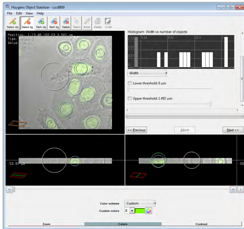
FIGURE 21.4. The Optimizing object detection screen in the Object Stabilizer.
